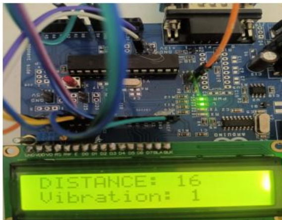
Fig 6 Illustration of distance and vibration detection
